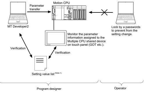
(Note-1): List of safety observation function parameter printed by print function of MT Developer2.
