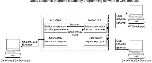
The following shows how to transfer safety observation function parameters and user safety sequence programs created by programming software to CPU modules.
