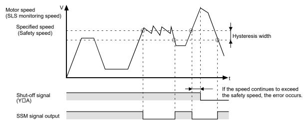
SSM signal output is constantly updated regardless of the safety observation error while the speed monitoring enabled signal is ON. SSM output is OFF when the speed monitoring enabled signal is OFF.
