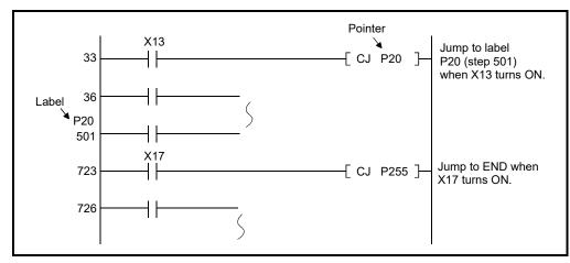
The pointer indicates the branch instruction (CJ, CALL) jump destination. The pointer number assigned at the jump destination head is called the label.
