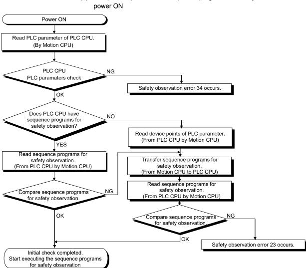
(a) Comparison procedure of sequence programs for safety observation at
