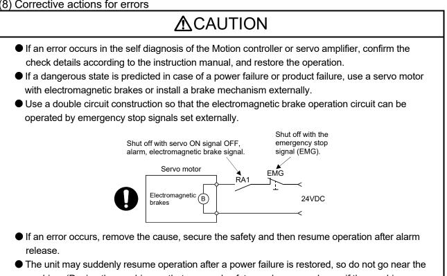
machine. (Design the machine so that personal safety can be ensured even if the machine restarts suddenly.)
