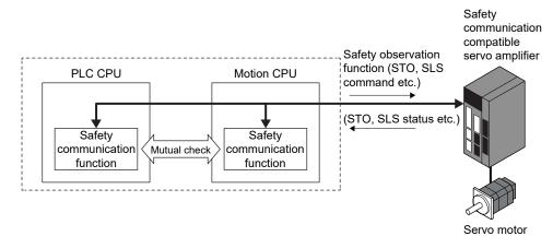
Safety information is communicated by SSCNETI/H between a Motion CPU and servo amplifier that support safety communication. Data is created and compared by the Motion CPU and PLC CPU. Safety communication function can only be used with SSCNETI/H communication. Safety communication function cannot be used with SSCNETI communication.
