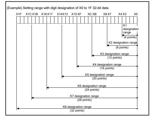
(3) When a digit is designated on the source (S) side The values that can be handled as source data will be as shown below.
