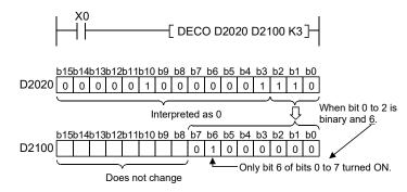
(Note-1): The D2100 bit 0 turns ON when the b0 to b2 of D2020 are 0. (Note 2): The D2100 details remain the same even if X0 turns OFF.
