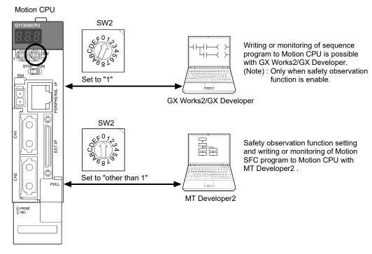
The connection destination can be selected from the PLC CPU or Motion CPU by Transfer Setup of programming software.
