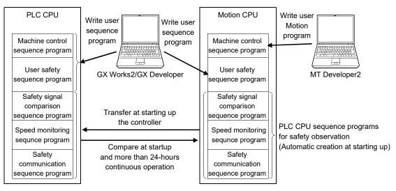
(2) Comparison of sequence programs for safety observation After the sequence program is transferred to PLC CPU, the Motion CPU reads
