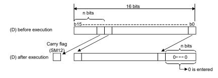
• Specify any of 0 to 15 as n. If the value specified as n is out of range, the remainder of n / 16 is used for rotation. (As n is BIN 16 bits unsigned value.) For example, when n=18, the contents are rotated two bits to the left since the remainder of 18 / 16 = 1 is "2".
