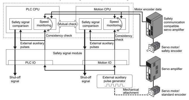
The system configuration for speed monitoring function is shown below.
