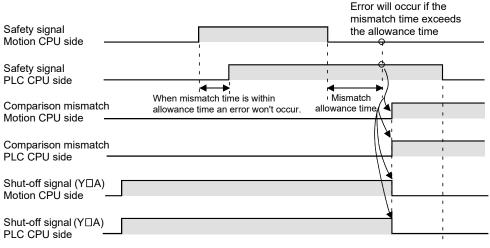
Shut-off signal will still be OFF even when the signals match after error detection.
