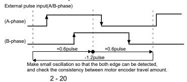
If the difference between value of motor encoder and external auxiliary pulse input occurs, "Safety observation error (error code: 121)" occurs, and the shut-off signal is turned OFF.
