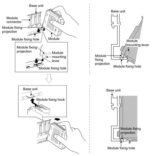
• When installing the module, always insert the module fixing projection into the module fixing hole of the base unit.
