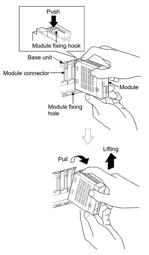
• When the module fixing screw is used, always remove the module by removing the module fixing screw and then taking the module fixing projection off the module fixing hole of the base unit.
