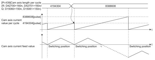
\*1 Because the coordinate where "input value = cam axis length per cycle" does not exist, the final coordinate is calculated from the line segment between the nearest two coordinates.
