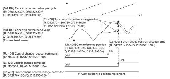
When "[Rq.406] Control change request command (R: M42408+16n/Q: M11688+10n)" is reset to OFF while executing the cam reference position movement command, operation is stopped midway. If the cam reference position movement command is executed again, the remainder travel value is not reflected, and the operation starts with "[Cd.408] Synchronous control change value (R: D42772+160n, D42773+160n/Q: D15132+150n,D15133+150n)" to be used again.
