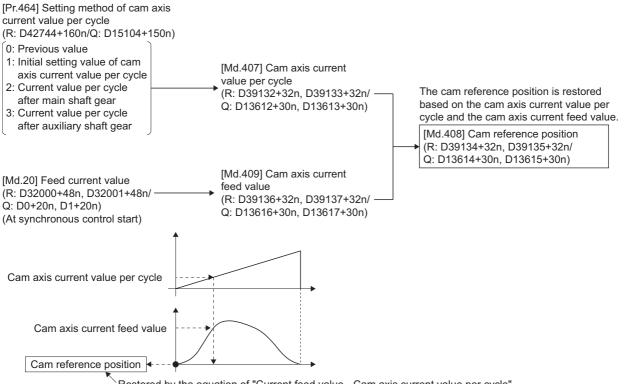
Restored by the equation of "Current feed value - Cam axis current value per cycle"
