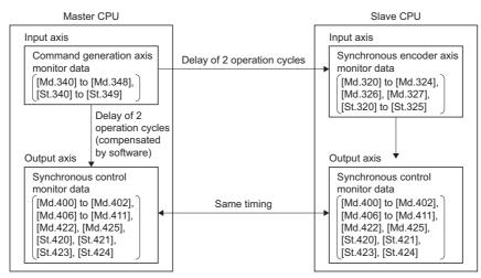
• To remove the delay time described above, using the phase compensation function of the output axis for the slave CPU and the master CPU, set a value that adds a delay compensation time of two operation cycles to the delay time inherent to the system. Refer to phase compensation on delay time of the input axis for delay time inherent to the system. (Is Page 166 Phase compensation on delay time of the input axis)
