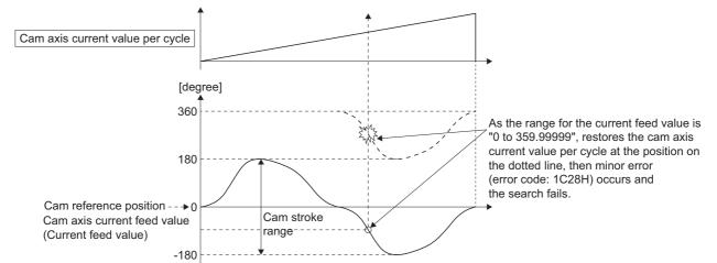
• In the case above, execute cam axis current value per cycle restoration within a cam stroke range exceeding 0 and less than 360[degree]
