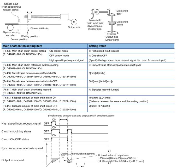
Slippage amount at clutch ON ...Distance between the ...Set as 20n sensor and the waiting position (100mm(3.94inch))
