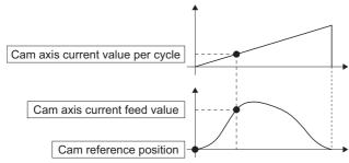
Select from 3 objects as follows in "[Pr.462] Cam axis position restoration object (R: D42742+160n/Q: D15102+150n)" which position is to be restored. ( Page 151 Cam Axis Position Restoration Method)
