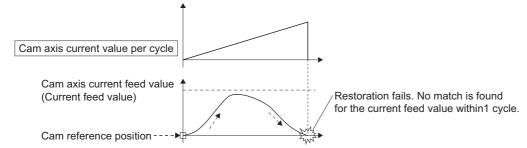
(2) When the unit is "degree" and cam axis current value per cycle restoration is executed in a cam stroke range that straddles 0
