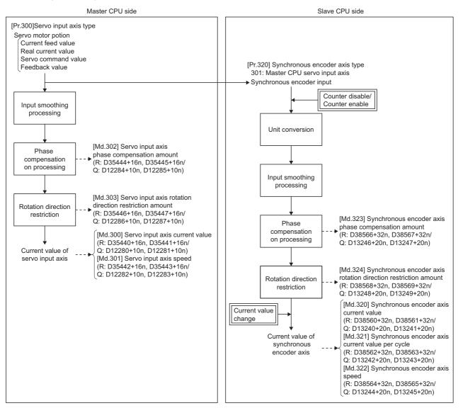
If "501: Master CPU synchronous encoder axis" in "[Pr.320] Synchronous encoder axis type" is selected The change amount of the input pulse to the synchronous encoder on the master CPU is transmitted to the slave CPU. Also, control by a current value change by "[Rq.320] Synchronous encoder axis control request (R: M42241+8n/Q: D14823+20n)", counter enable, and counter disable, are not reflected in the change amount that is transmitted.
