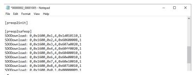
**4.** Add a command to the [preop2safeop] section of the CUI file. The contents of the command specify the time difference between UTC and Japan in minutes. (Example: 9 hours x 60 minutes = 540 minutes)
