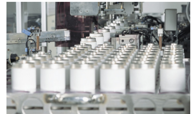
Fitting of a guide, measurement of vacuum degree and bellows force are carried out automatically
