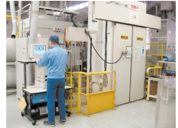
Automatic conditioning and electrical testing device
