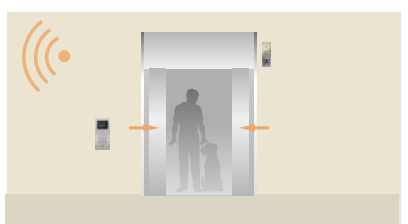
An announcement identifying the car assigned (e.g. "Elevator A") is played and repeated until just before the car door begins to close.
