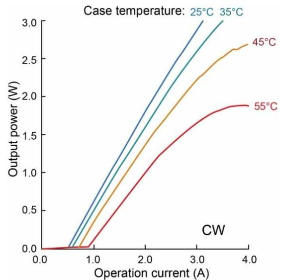
Fig. 3 Output power – Current characteristics
