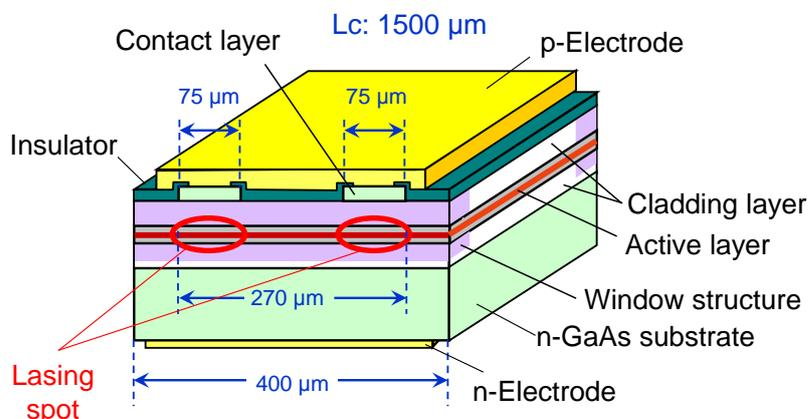
Fig. 1 Device structure of the red LD
