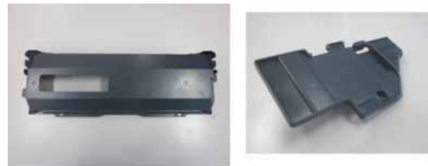
Fig. 3 Example of the parts of a room air conditioner using flame-resistant recycled PS
