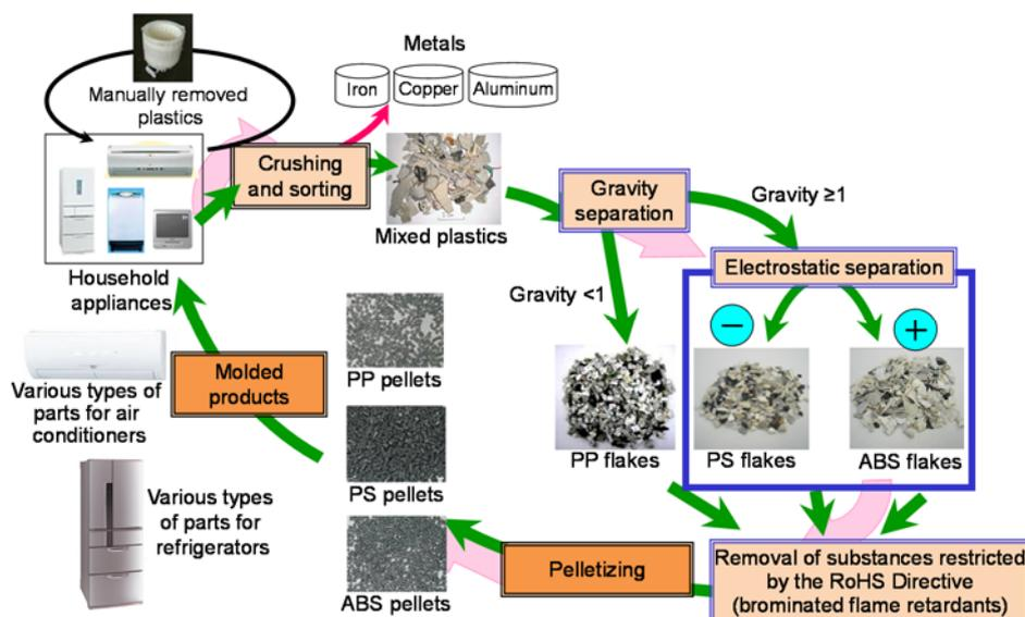
Fig. 1 Flow chart of closed-loop plastic recycling technologies
