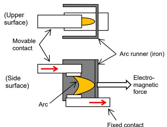
Fig. 1 Schematic diagram of arc attraction by arc runner
