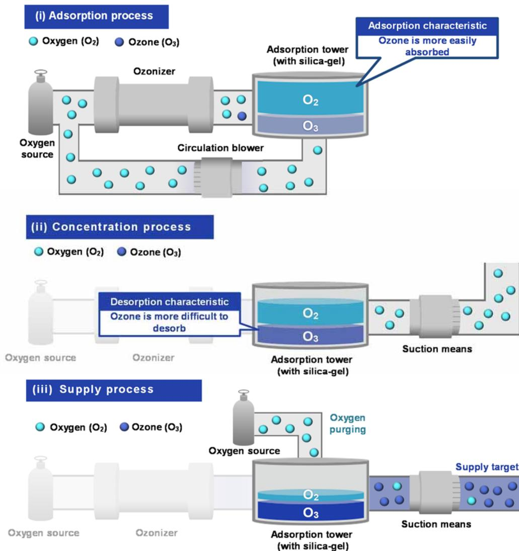
Fig. 3 Operation flow of ozone concentration storage device
