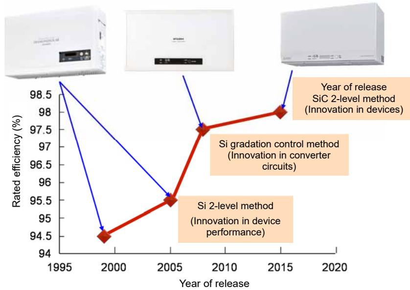
Fig. 4 Improvement of power conversion efficiency
