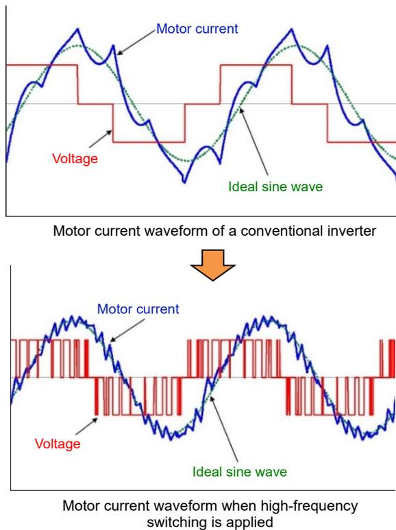
Fig. 5 Motor loss reduction using high-frequency switching
