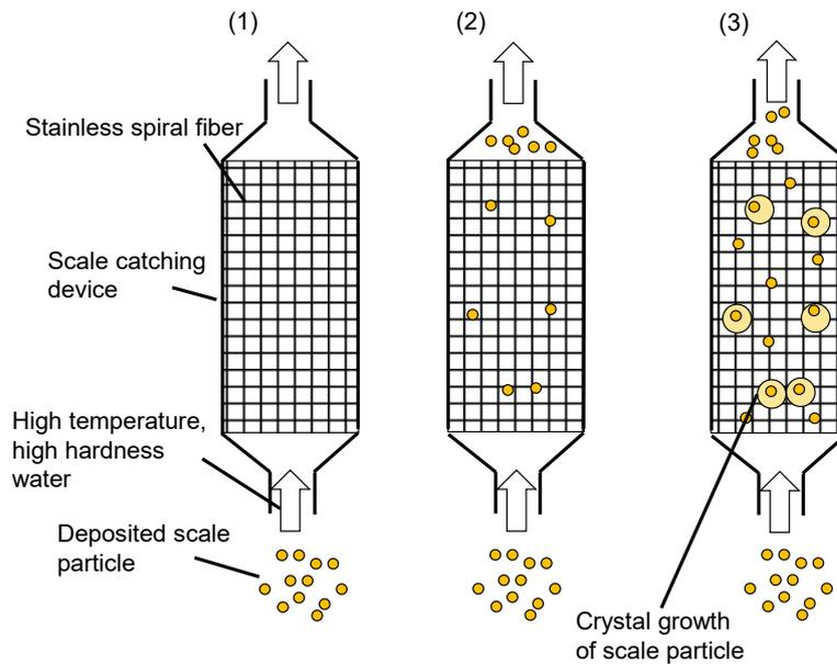
Fig. 5 Concept of scale capture process in the scale catching device
