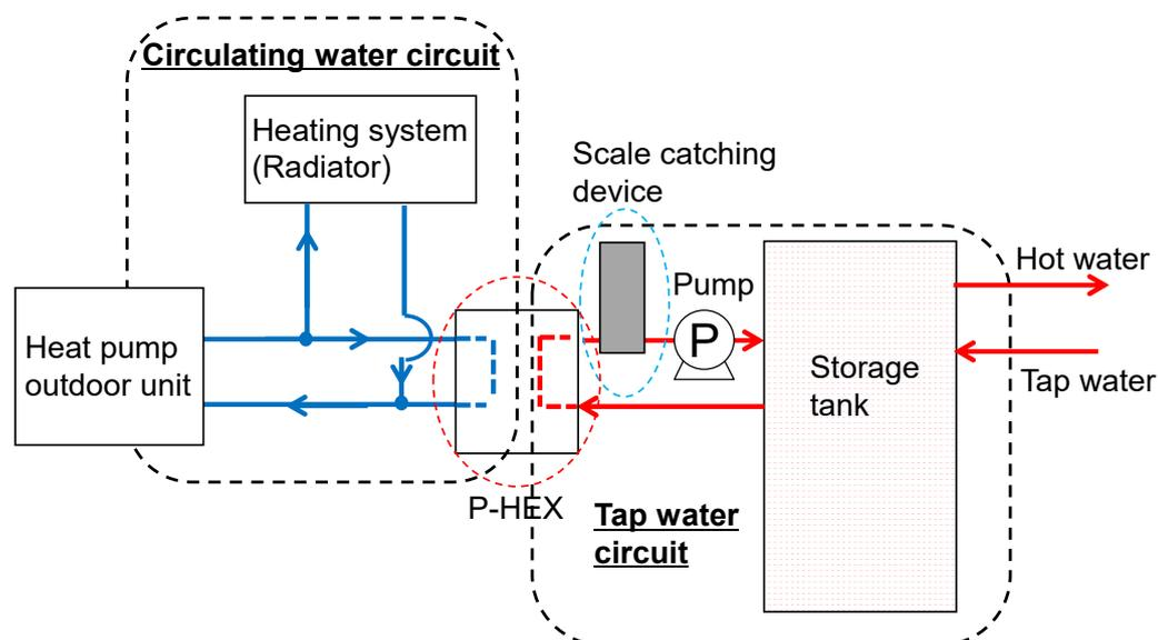
Fig. 1 Schematic of the 2014 ATW system
