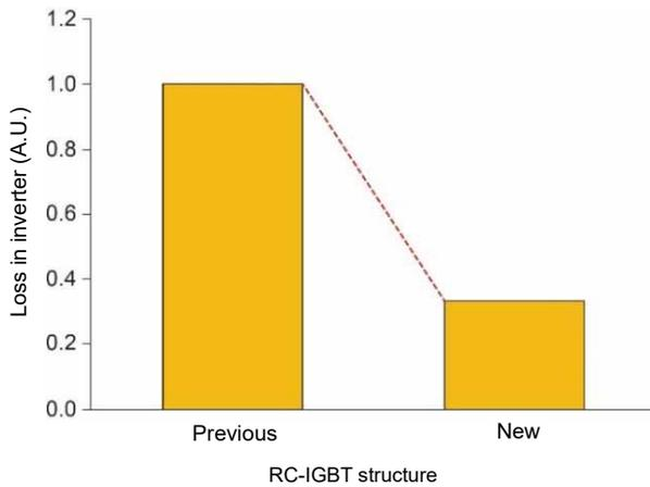
Fig. 6 Comparison of total inverter loss between previous RC-IGBT and second-generation RC-IGBT
