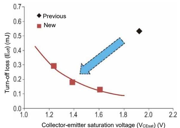
Fig. 4 Trade-off relationship between  $V_{CEsat}$  and  $E_{off}$
