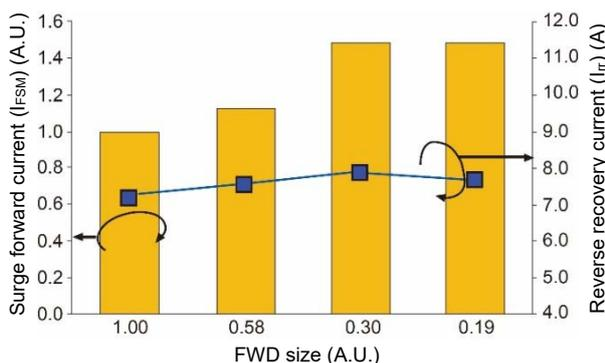
Fig. 3 FWD size dependence of  $I_{FSM}$  and  $I_{rr}$
