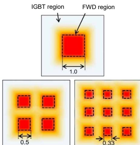
Fig. 2 Design concepts of FWD layout: optimizing the thermal distribution
