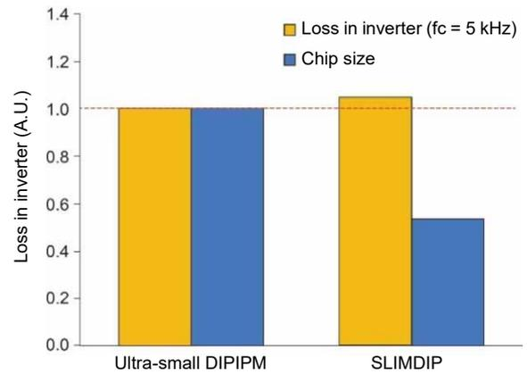
Fig. 7 Comparison of total inverter loss and chip size between the latest DIPIPM and SLIMDIP
