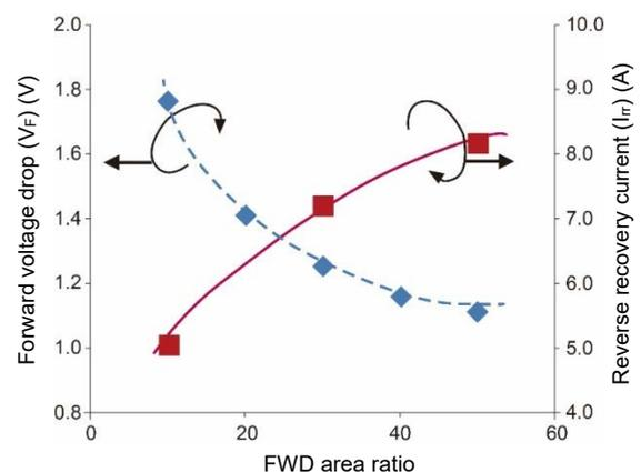
Fig. 1 FWD area ratio dependence of  $V_F$  and  $I_{rr}$
