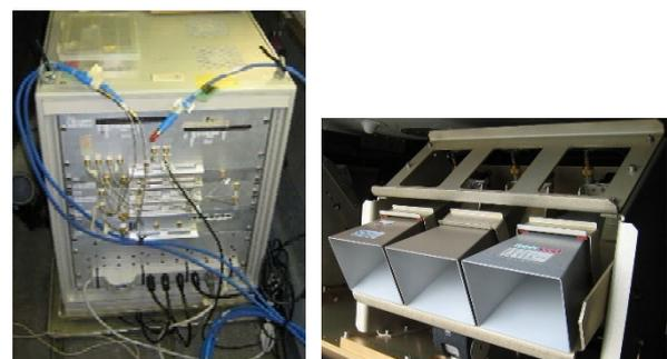
Fig. 5 Ku-band airplane SAR system
