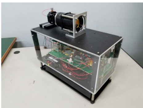
Fig. 1 Schematic block diagram and external view of the mobile Doppler lidar
