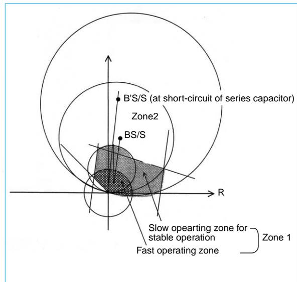
Fig. 1 Operating zone setting of AS/S distance relay element
