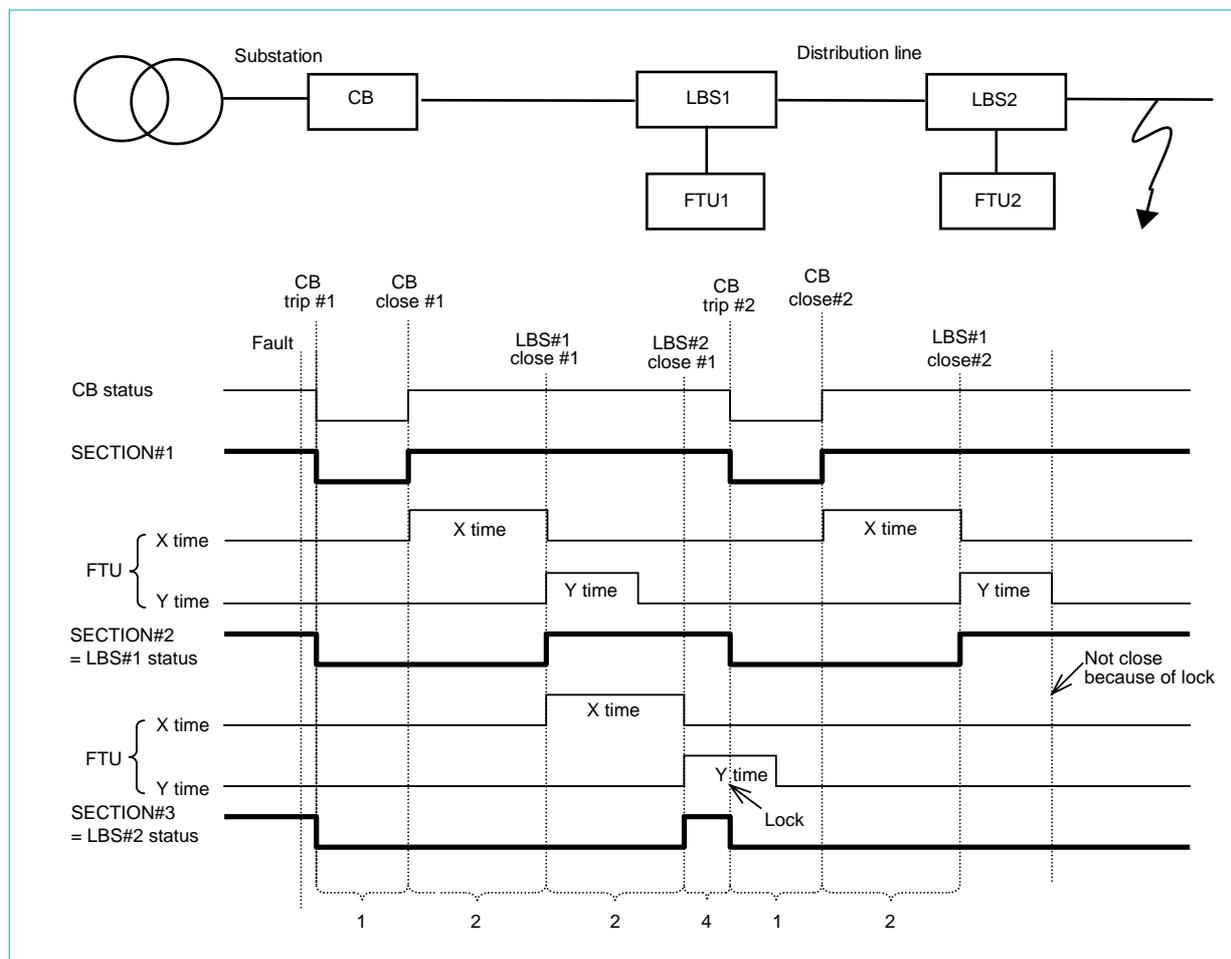
Fig. 4 Self-closing diagram
