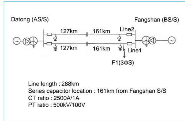
Fig. 4 Line system diagram between Datong and Fangshan
