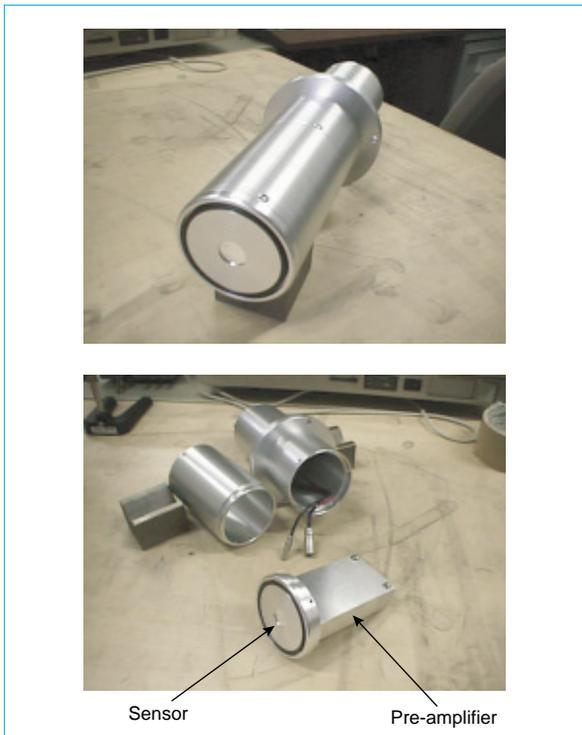
Fig. 2 Semiconductor beta-ray gas monitor
