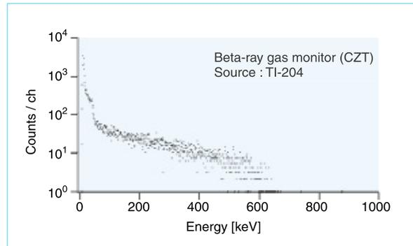
Fig. 3 Beta-ray gas monitor energy spectrum
