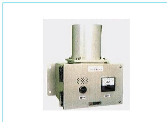
Fig. 1 External view of the area monitor
