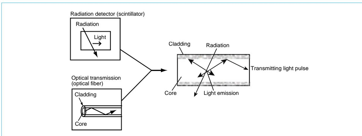
Fig. 2 Principle of detection
