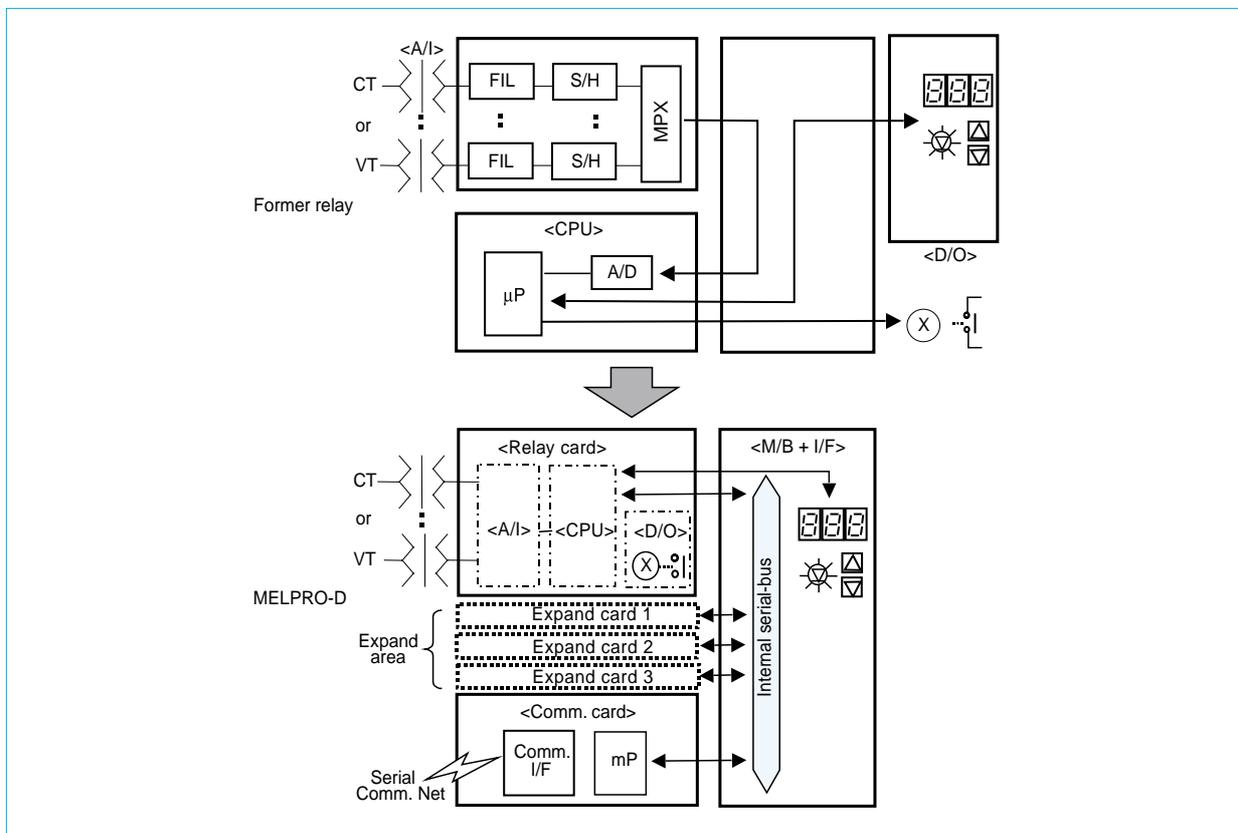
Fig. 2 Internal block diagrams of former and MELPRO-D relays
