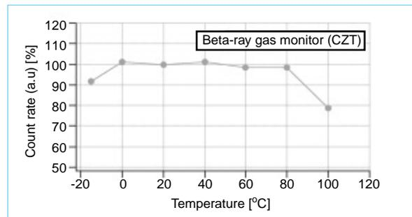
Fig. 4 Beta-ray gas monitor temperature characteristics
