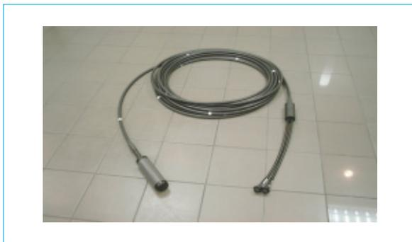
Fig. 1 Detector of the fiber-optic radiation sensing system
