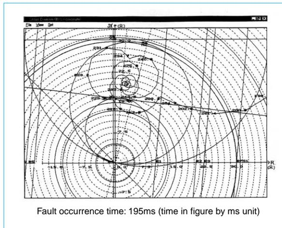
Fig. 3 Impedance locus at A S/S relay (at F1 3 $\Phi$ S fault of Fig. 4)
