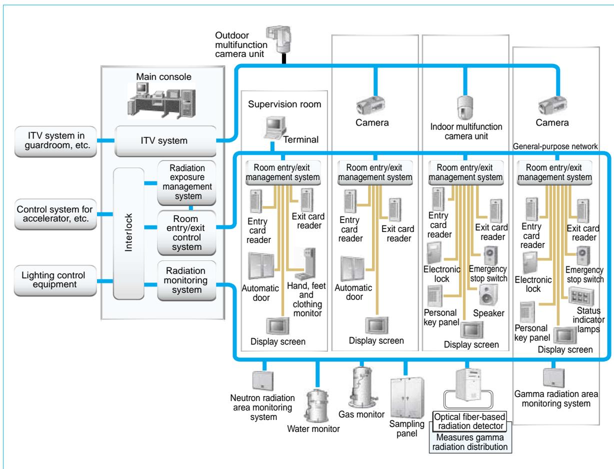
Fig. 1 Radiation-management computer system
