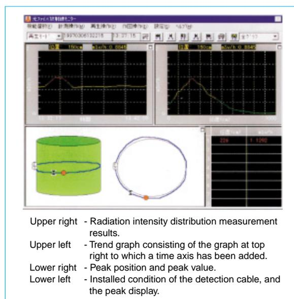
Fig. 4 Example of display screen
