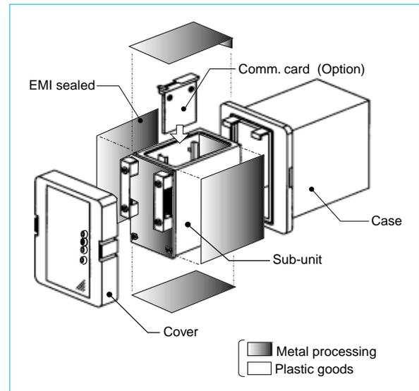
Fig. 3 Typical unit structure
