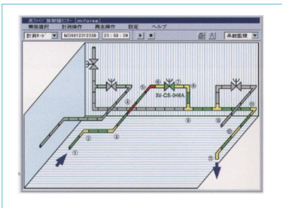
Fig. 5 Example of a screen showing the radioactive waste resin being transferred
