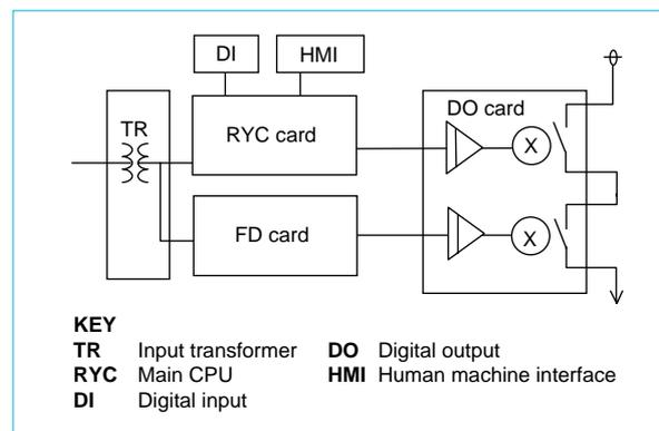
Fig. 4 Hardware-independent fail-safe function
