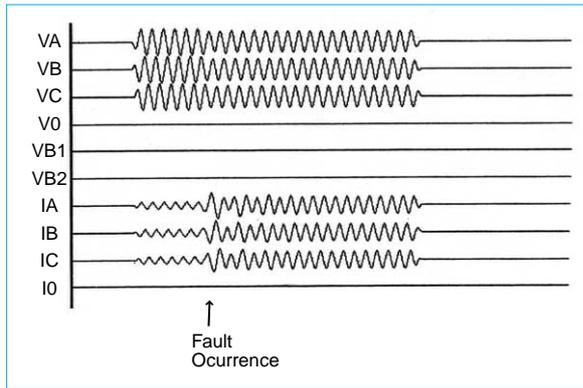
Fig. 2 Fault waveform of voltage and current saved on the AS/S relay (at F1 3 $\Phi$ S fault of Fig. 4)
