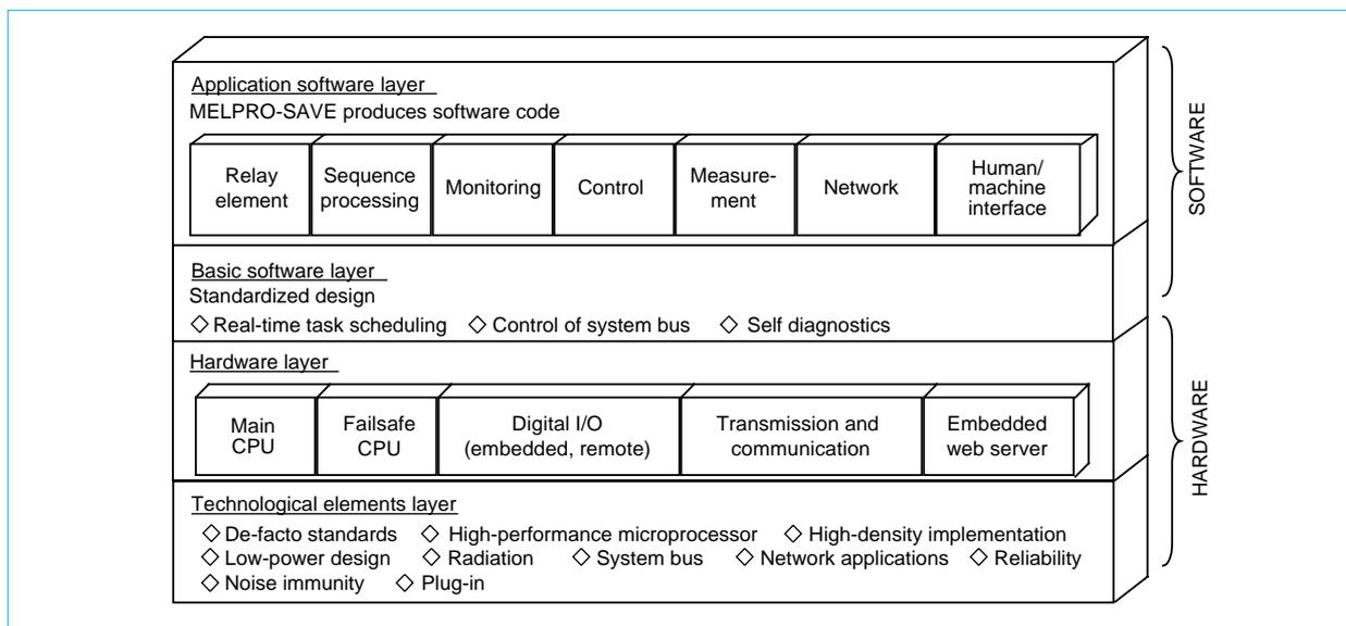
Fig. 1 Architecture of basic technological elements used in MELPRO-C relays
