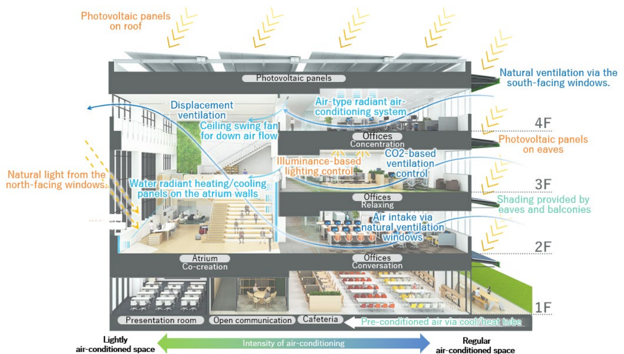
Hierarchical building design that incorporates “Passive” and “Active” design approaches
