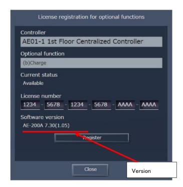
•How to check versions on the screens of AG-150A-A, AG-150A-J, AE-200A, AE-200E, AE-50A, AE-50E, TE-200A, and TE-50A
