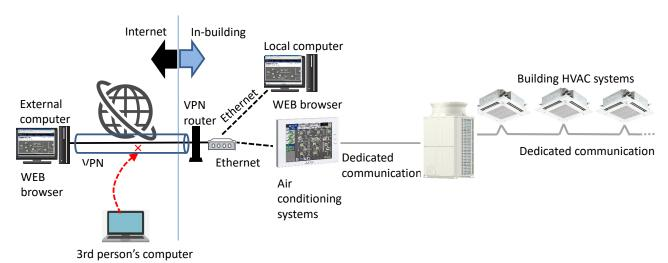
**System Example 3**: A configuration using air conditioning systems which is accessible from external computers without VPN (improper configuration)
