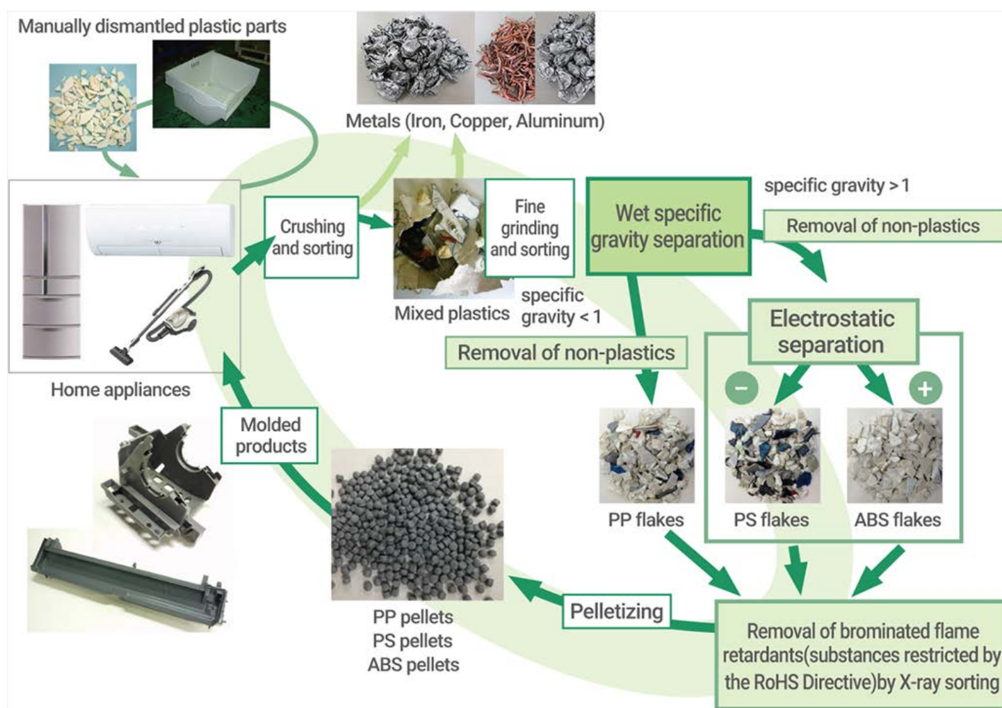
Flow chart of Mitsubishi Electric Group closed-loop plastic recycling
