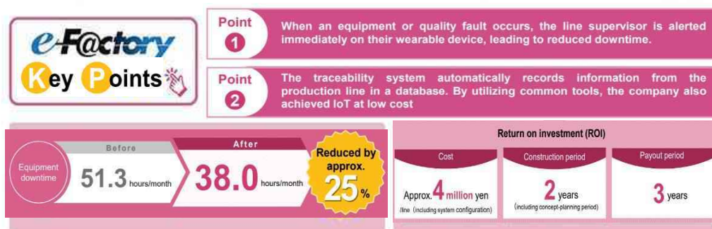
ROI example of a case where equipment downtime was reduced by 25% by using low-cost IoT
