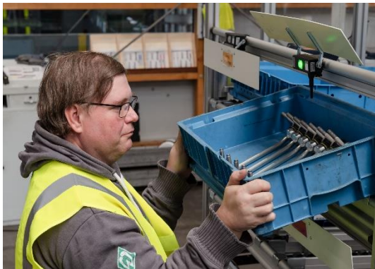
Fig. 5: A physical access barrier to the parts bin is provided by means of an intelligent door flap mechanism (pick-to-door). Simultaneously, an illuminated push button on the bin prompts removal of the part, which is acknowledged by pressing the button (pick to light).
