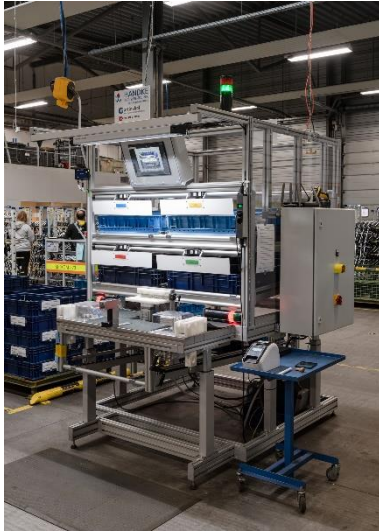
Fig. 1: Each of the new manual workplaces consists of an aluminium profile frame fitted with hydraulic height adjustment for adapting to different ergonomic requirements, plus illumination and workpiece receptacle.
