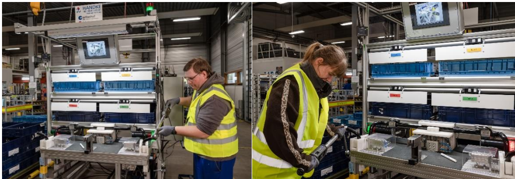
Figs. 2+3: Thanks to the poka-yoke controller, existing technology – like a digital torque wrench in this case – was integrated into the error-free process without problems.
