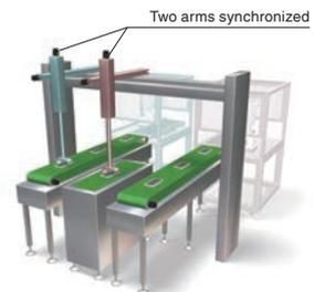
The two arms can avoid interference by synchronizing with each other, shortening the cycle time.
