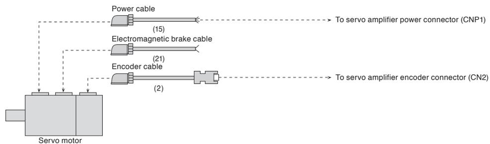
Notes: 1. Cables for leading two different directions may be used for one servo motor.
