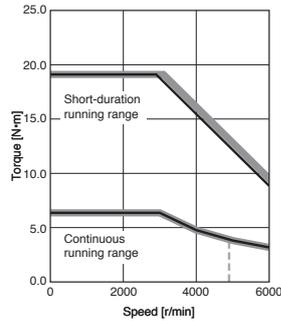
Notes: 1. Torque drops when the power supply voltage is below the specified value. - - - - : A rough indication of the possible continuous running range for 3-phase 323 V AC
