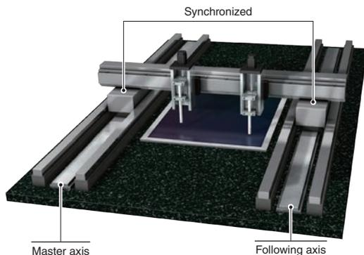
Motion Control Software enables tandem operation where the same commands can be outputted to master and following axes.
