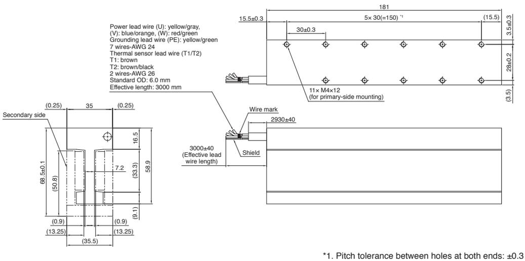
Notes: 1. Power, grounding, and thermal sensor lead wires do not have a long bending life. Fix the lead wires led from the primary side (coil) to a moving part to prevent the lead wires from repetitive bending.
