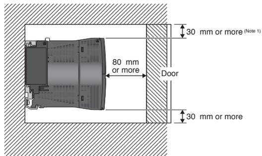
Notes: 1. Provide clearance of 30 mm or more when the height of a wiring duct is 50 mm or less. In other cases, provide clearance of 40 mm or more.
