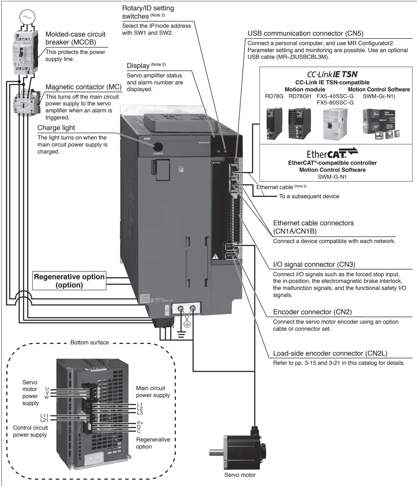
Notes: 1. The connection with the peripheral equipment is an example for MR-JET-700G4-HS(N1) servo amplifiers. Refer to "MR-JET User's Manual" for the actual connections.
