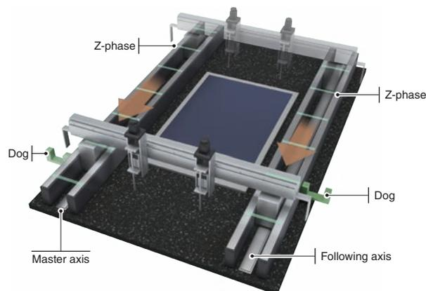
After the master and following axes pass their respective dogs, the gantry home position return stops both of the axes at the Z-phase of the master axis. This method enables two or more axes to execute home position return simultaneously, supporting gantry systems.
