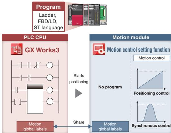
A PLC CPU program starts operation of the Motion module, eliminating the need for users to create another program for the Motion module, reducing programming burden.
