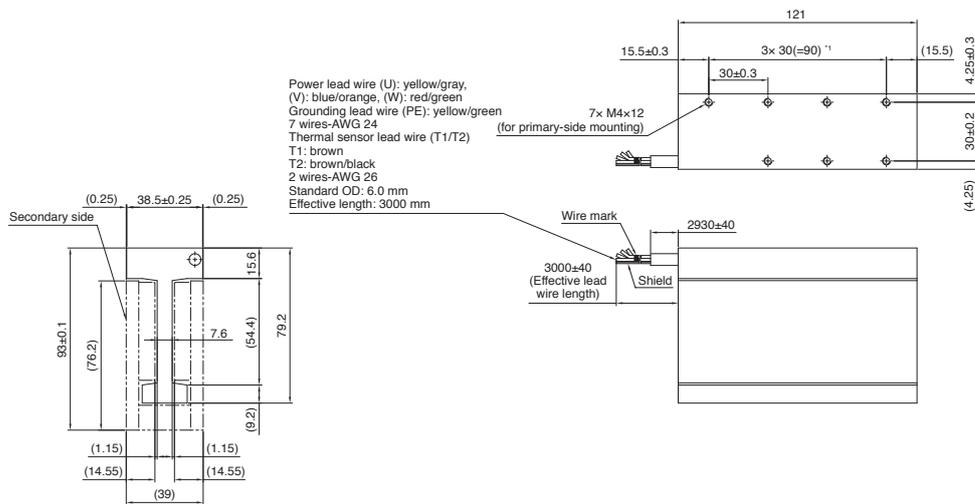
\*1. Pitch tolerance between holes at both ends:  $\pm 0.3$
