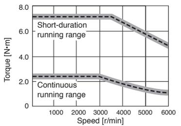
Notes: 1. Torque drops when the power supply voltage is below the specified value.
