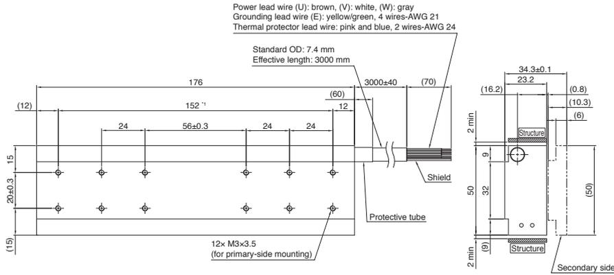
\*1. Pitch tolerance between holes at both ends:  $\pm 0.3$  [Unit: mm]
