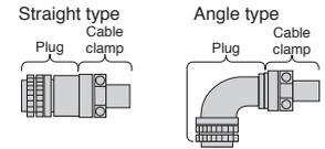
Power connector for HK-FN (1.0 kW to 3.0 kW) series/HK-SN series
