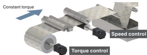
**Continuous Operation to Torque Control**
