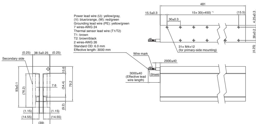
\*1. Pitch tolerance between holes at both ends: ±0.3 [Unit: mm]
