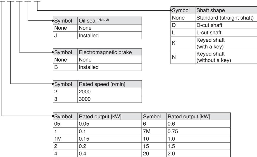
●HK-FN series (high inertia, small/medium capacity)
