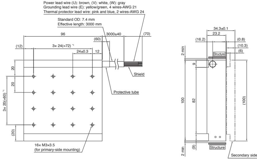
\*1. Pitch tolerance between holes at both ends: ±0.3 [Unit: mm]
