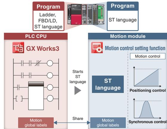
Motion modules can execute operations in place of the PLC CPU. This reduces the operation burden on the PLC CPU and results in a shorter cycle time.
