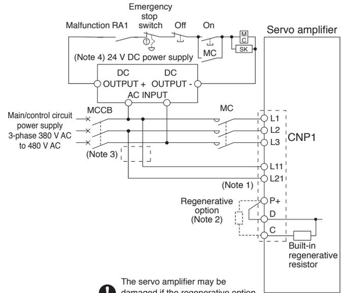
⚠ The servo amplifier may be damaged if the regenerative option is incorrectly connected.
