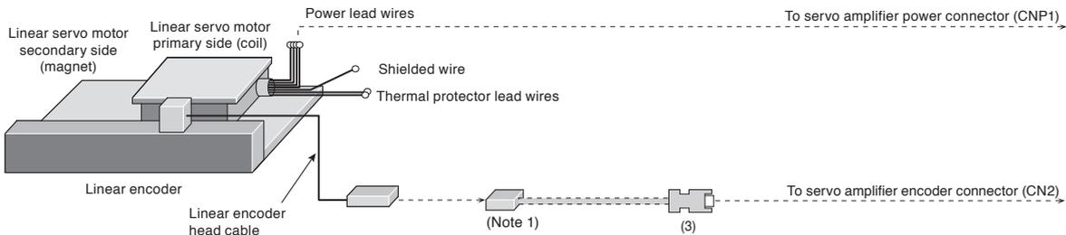
Notes: 1. Contact the relevant linear encoder manufacturers for connectors to connect with the head cables.
