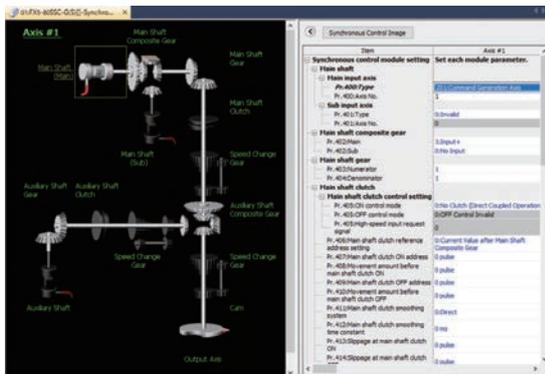
Synchronous control is executed by setting parameters of the input axis, output axis, gear, and clutch for synchronous control and turning on the synchronous control start signal.
