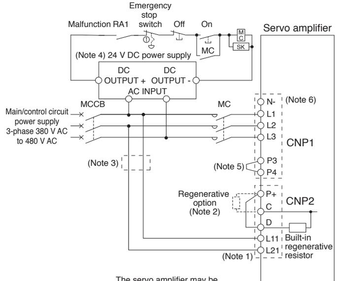
⚠ The servo amplifier may be damaged if the regenerative option is incorrectly connected.
