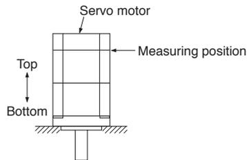
\*4. Refer to the diagram below for the shaft-through portion.
