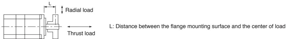
\*3. V10 indicates that the amplitude of the servo motor itself is  $10\ \mu\text{m}$  or less. The following shows mounting orientation and measuring position of the servo motor during the measurement:
