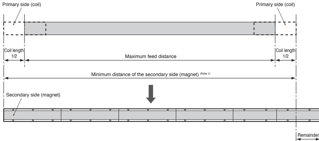
Notes: 1. Pitch tolerance between any two holes must be within  $\pm 0.2$  mm. When two or more secondary sides (magnets) are mounted lined up, there may be a gap between each block, depending on the mounting method and the number of the blocks.
