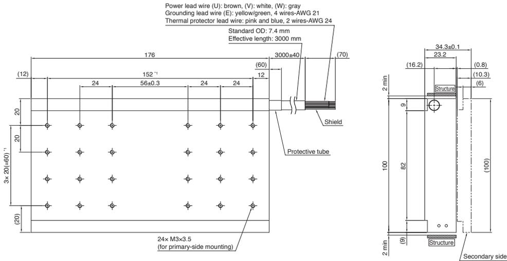
\*1. Pitch tolerance between holes at both ends: ±0.3 [Unit: mm]
