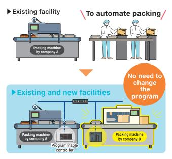
Connect to an integrated PLC for even better monitoring of production.
