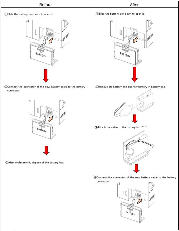
$\label{eq:note1} \textbf{[Note1]} \ \text{When attaching to the battery box, please insert two wires one by one.}$
