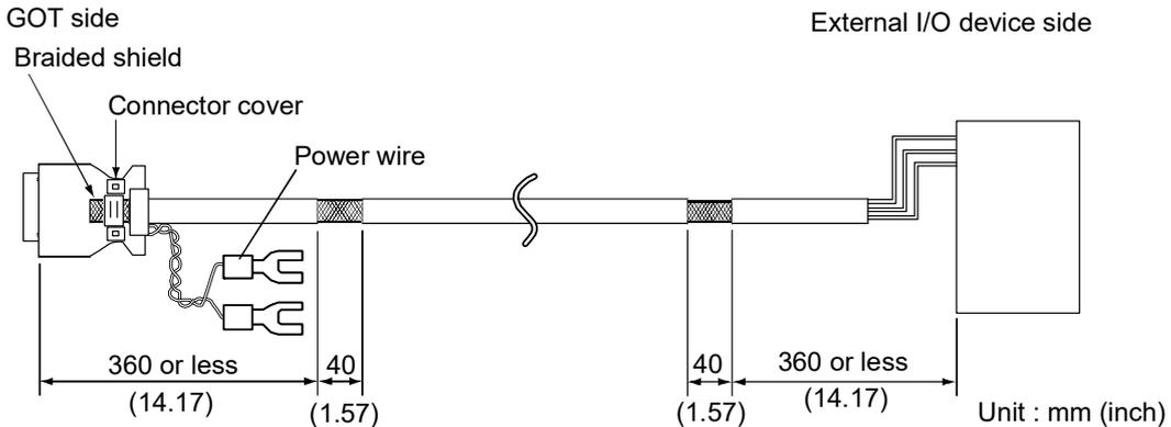
(f) Connection of third party PLC, microcomputer, temperature controller, inverter, servo amplifier, CNC, MODBUS/RTU or MODBUS/TCP
