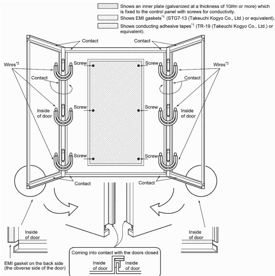
\*1 Do not apply coating to the parts where EMI gaskets and conducting adhesive tapes are to be attached.
