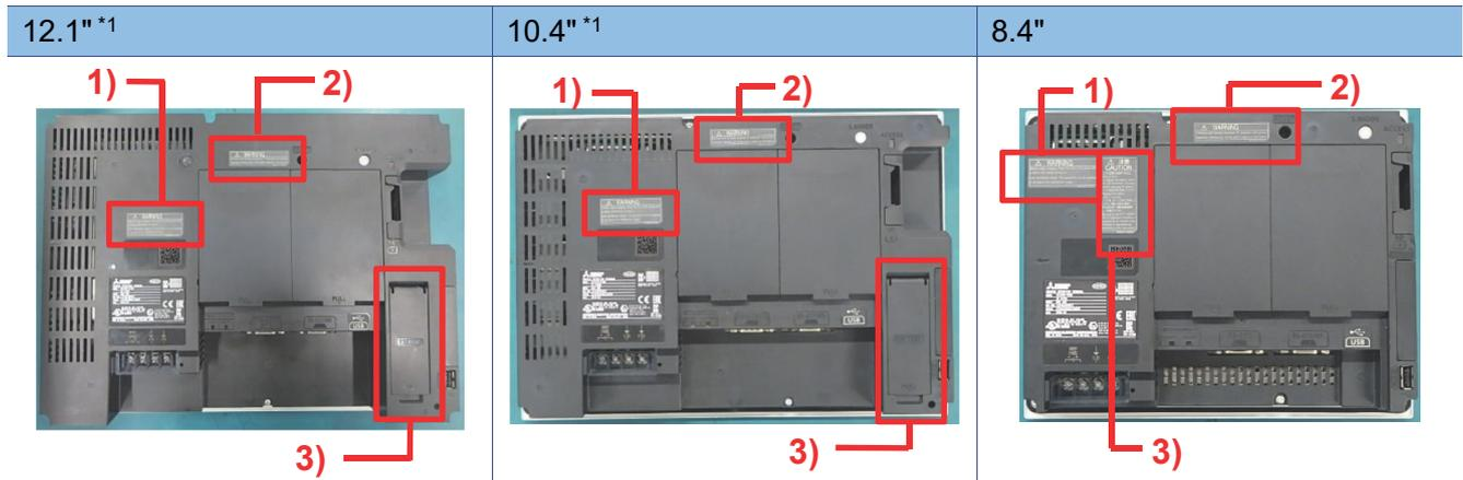
\*1 The 12.1" or 10.4" GOT has the battery caution plate under the battery cover.
