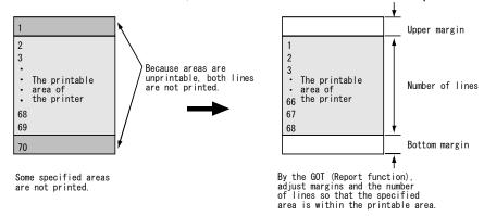
When some of lines are not printed for the report function of the GOT, configure the printer setting with no trimming. Doing so may print the lines correctly.
