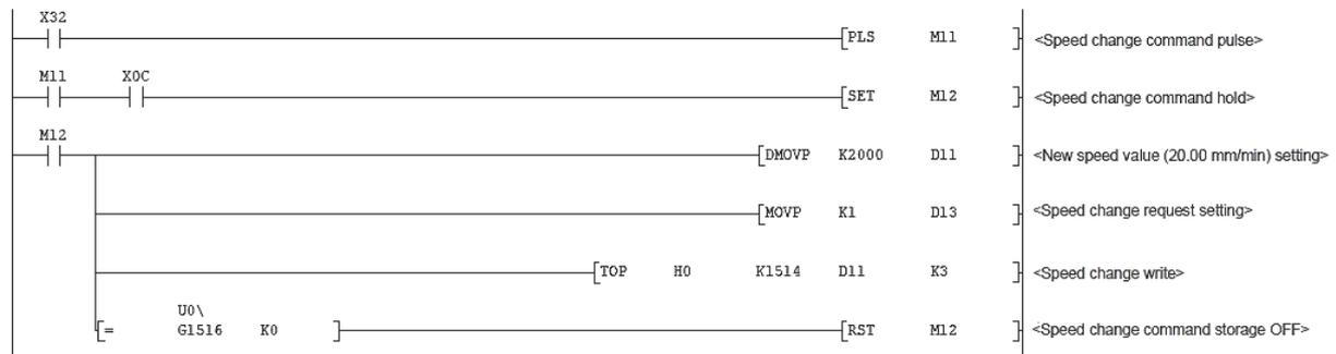
■ Speed change using override function (QD75 additional function)
