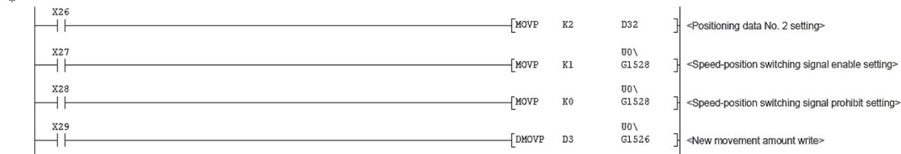
**■ Position-speed switching operation start data No. setting (QD75 additional function)**
