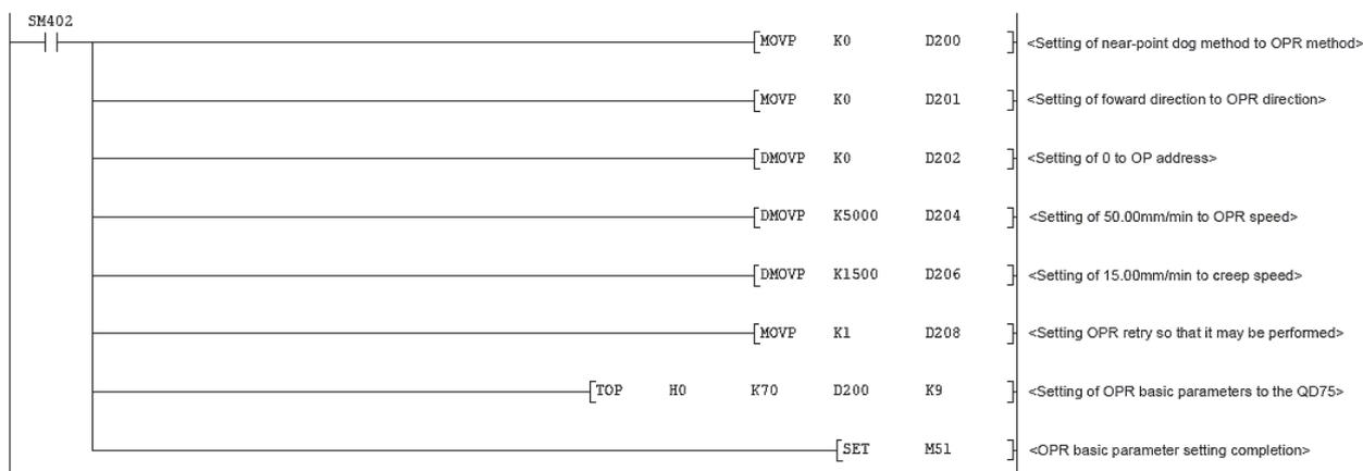
Speed-position switching control parameters setting (only when speed-position switching control function is used)
