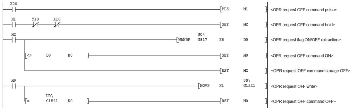
■ External command function valid setting (only when external command function is used)
