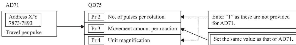
When using the error compensation function of the AD71, refer to the following to set "No. of pulses per rotation", "Movement amount per rotation" and "Unit magnification".
