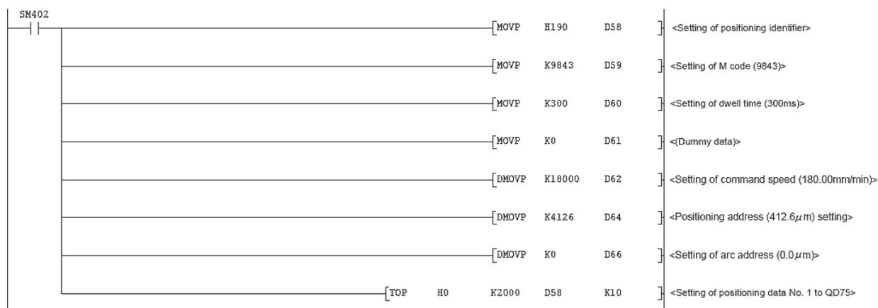
**■ Block start data setting (only when block start function is used)**
