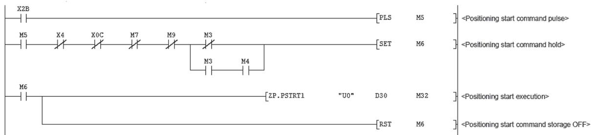
**Start using positioning start signal**
