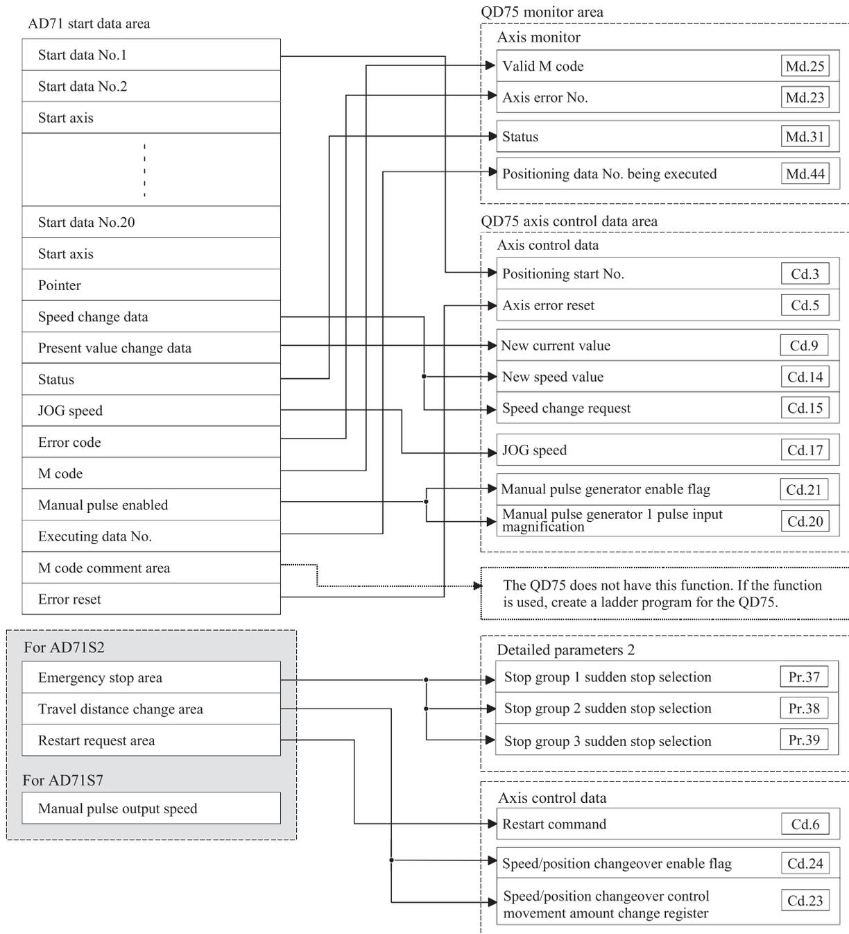
To enable the continuous positioning using the AD71 pointers, use the block start function.
