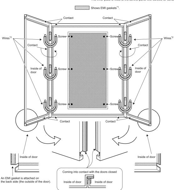
Shows an inner plate (galvanized at a thickness of 10µm or more). The inner plate is fixed to the control panel with screws for conductivity.
