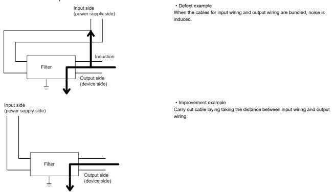
• Connect the noise filter's ground terminal to the control panel with the shortest possible cable (approx. 10cm).
