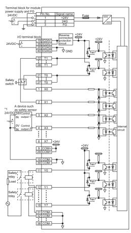
\*1 The power supply of 24VDC can be applied from the COM+ terminal.
