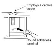
The round solderless terminal used for the existing model cannot be used for the CC-Link IE TSN remote I/O module with safety functions of the alternative model.
