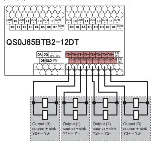
Since the double output of source and sink is not available, use the double output of source and source.
