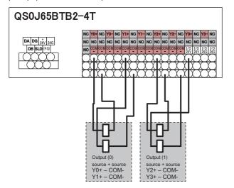
When the double output of source and sink is used, 4 points can be used. (Example) When the double output of source and sink is used
