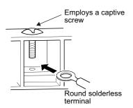
The round solderless terminal used for the existing model cannot be used for the CC-Link IE TSN remote I/O module with safety functions of the alternative model.
