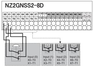
The 4 points in the latter half are connected to NZ2GNSS2-8D of the second station.
