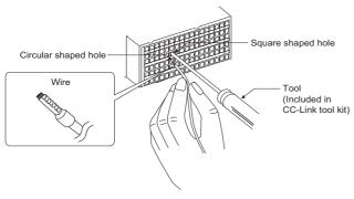
The bar solderless terminals used for the existing model cannot be used for the CC-Link IE TSN remote I/O module with safety functions of the alternative model.
