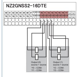
When the double output of source and sink is used, 4 points can be used. (Example) When the double output of source and sink is used
