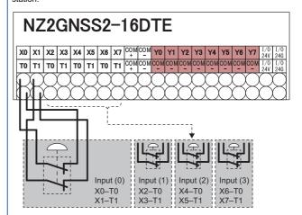
The 8 points in the latter half are connected to NZ2GNSS2-8D of the second station.
