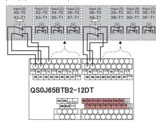
Double input: 4 points maximum, single input: 8 points can be used. (Example) When the double input is used
