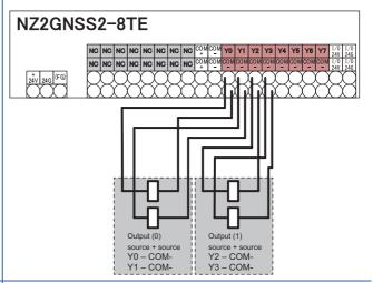
Since the double output of source and sink is not available, use the double output of source and source.
