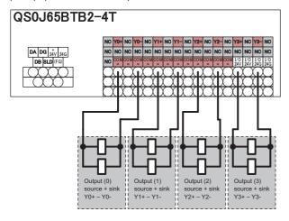
When the double output of source and source is used, 4 points can be connected.
