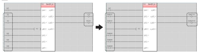
M1 is used to communicate the data between a standard program and safety program. Change the device to a standard/safety shared label.
