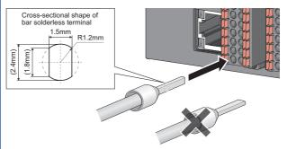
Use the recommended bar solderless terminals depending on the wire diameter.
