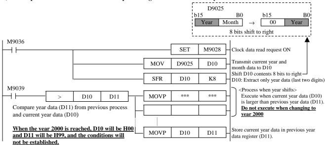
\* With this circuit, since the year data is two digits when shifting from the year 1999 to the year 2000, the size comparison conditions will not be established, and the target process will not be executed.
