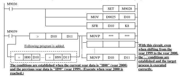
(Note) With the above circuit example, it is presumed that D10 and D11 are latch-designated, and the current year data is set in the previous year data D11 through initialization by another circuit.
