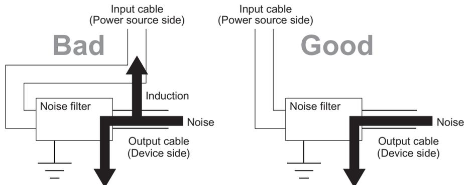
Installing the input and output cables together will cause noise induction.
