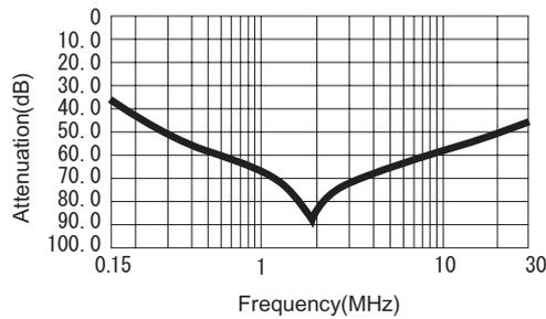
**Fig.2. Damping characteristics of noise filter**
