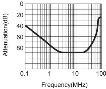
**Fig.2. Damping characteristics of noise filter for AC powered main unit**
