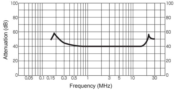
**Fig. 3. Damping characteristics of noise filter[2]**
