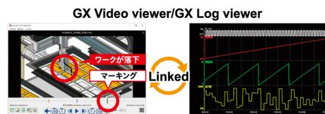
Video data recorded by the network camera and device data recorded by PLC can be linked for debugging. Since device numerical data matched with video playback can be checked, work efficiency is greatly increased.
