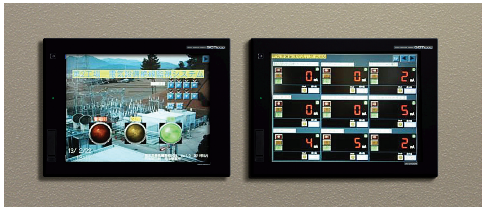
Main display screen (left) and individual monitoring results display screen (right) on the GOT. Values exceeding the set threshold values light up in yellow or red.
