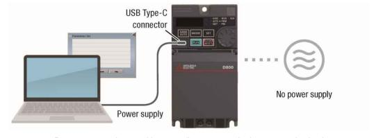
Parameters can be set without needing to power the inverters main circuit
