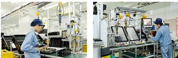
Cellular manufacturing facility producing PLCs and GOT HMIs
