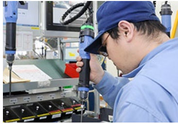
Lights on each screwdriver come on in the order in which they should be used
