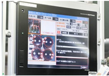
The display unit shows details of screw locations and sequence to prevent mistakes
