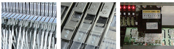
Components to be fitted are supplied on a reel. The equipment picks up the component from the tape by suction and fits it onto the board
