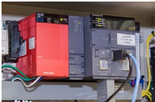
The C Controller for the production volume display device gets planned and actual volumes from the database via LAN, then compares the two on the display to reveal any delays in real time
