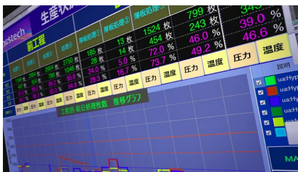
Lincstech visualized its real-time production status using Mitsubishi Electric's GENESIS64™ SCADA software.
