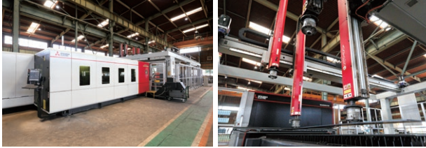
The automation of laser cutting operations through the combination of the GX-F60 and ASTES4 improved work efficiency and reduced the physical workload for operators.
