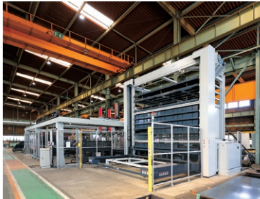
The introduction of the ASTES4 handling system means heavy steel sheets and processed products no longer need to be manually moved and stacked, reducing potential operational risks. “Increased safety is another major benefit,” says Komaya.
