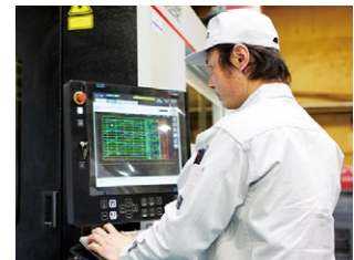
The control panel of the laser processing machine. The optional MEL'S AR function makes operation intuitive.
