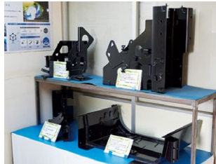
These components for construction machinery are formed through a combination of laser processing, bending, and welding. Laser processing is increasingly important for high-mix, low-volume manufacturing.
