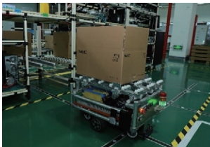
The AGV was developed in-house using a Mitsubishi Electric PLC. Routes can be changed by GOT touchscreen operation.
