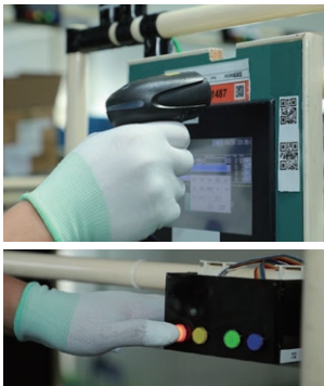
The digitalized picking process. When information about the model to be produced is scanned with a barcode reader, LEDs indicate which shelves the parts should be picked from. After picking the parts, the LEDs are turned off to prevent the same parts being picked twice.
