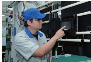
The AGV was developed in-house using a Mitsubishi Electric PLC. Routes can be changed by GOT touchscreen operation.
