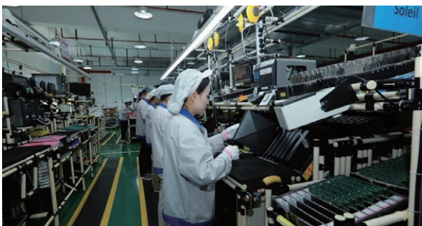
Router production line at the Suzhou plant. 58 models are assembled on ten mixed-flow lines.
