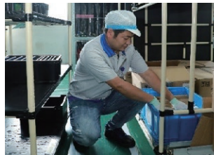
The digitalized picking process. When information about the model to be produced is scanned with a barcode reader, LEDs indicate which shelves the parts should be picked from. After picking the parts, the LEDs are turned off to prevent the same parts being picked twice.
