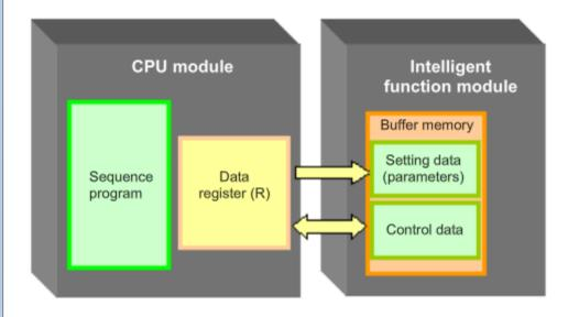
Example of setting data (in the case of D/A converter module)
