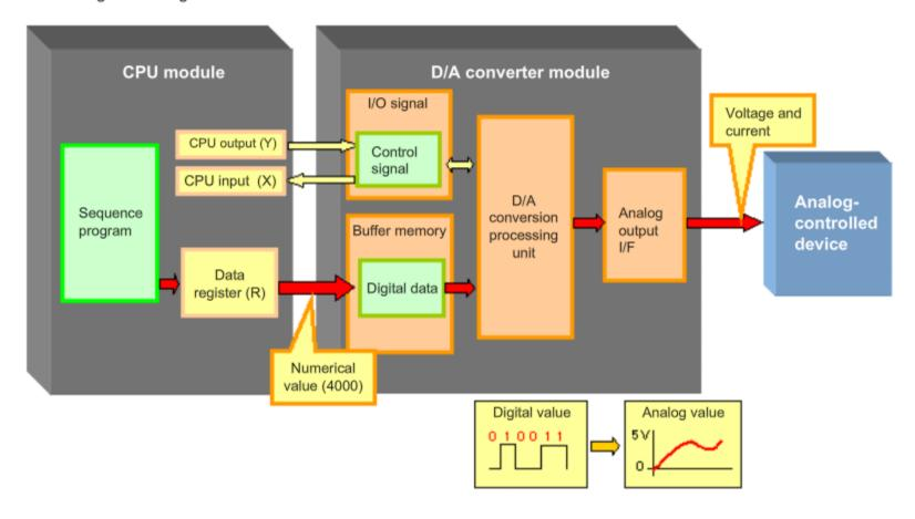
The D/A converter module converts digital data set by a sequence program into analog data (voltage or current), and then outputs them to external devices. The details are explained in Chapter 2.
