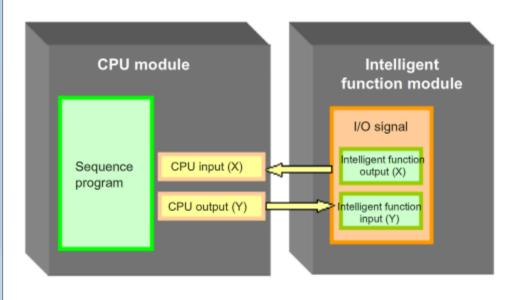
X signals inform the CPU module about the status of intelligent function modules with ON/OFF signals.
