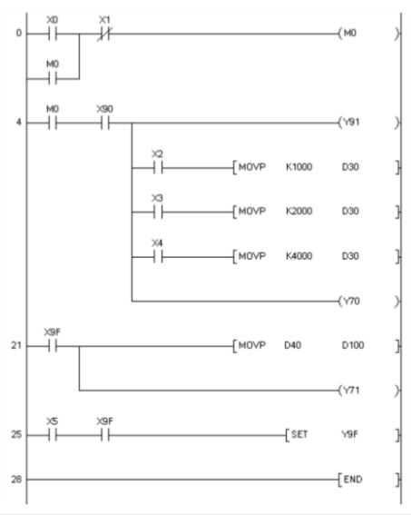
When X0 is ON, M0 is self-held (during D/A conversion). When X1 is ON, self-holding is cancelled.
