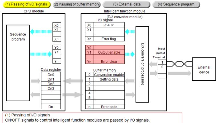
"X" is a signal received by the CPU module side and "Y" is a signal transmitted by the CPU module side as a command.
