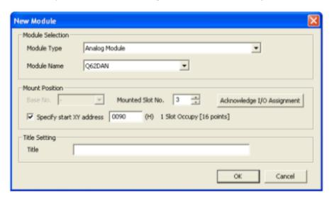
Mounted Slot No. and Start XY address can be changed after being set.
