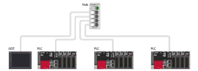
PLC CPU devices are monitored by connecting the GOT to the built-in RS-232 or RS-422 interface of the PLC CPU.  $^{\star1}$
