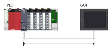
When the RS-232 is used Max. connection length: 3 m When the RS-422 is used Max. connection length:  $30.5 \text{ m}^{*2}$
