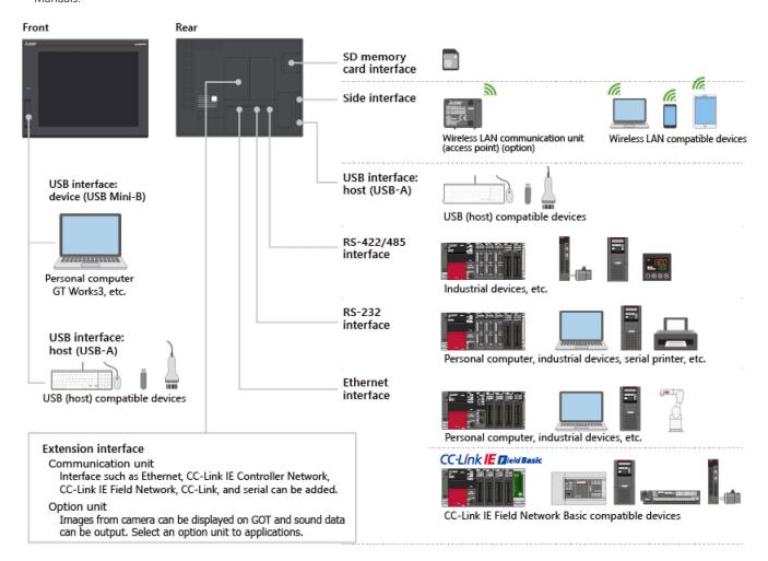
The GOT can be connected to the PLC using various types of connection to monitor the PLC. Connection types are selectable according to the system configuration and application.
