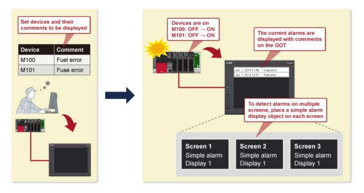
Set target devices for alarm display. The alarm display (user) object collects alarms of the set devices by monitoring them. The object displays the collected alarms (currently occurring alarms and past alarms).
