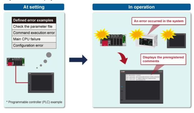
There are two ways to display the user alarm display and the system alarm display. One is to display the currently occurring alarms only, and the other is to display the currently occurring alarms and the alarm history as well.
