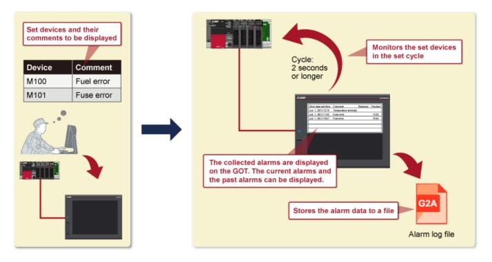
A system alarm display object displays the comments prepared in the system on the GOT when alarms occur. The object monitors the GOT, controller, and network and displays the codes and messages of the errors when they occur.
