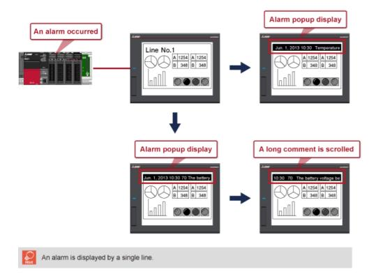
The user alarm function displays the comment for one alarm separately in the upper alarm comment, middle alarm comment, or basic alarm comment. In the basic alarm, the detailed information such as the cause of the alarm and corrective actions can be displayed in the comment window, the base screen, and the window screen.
