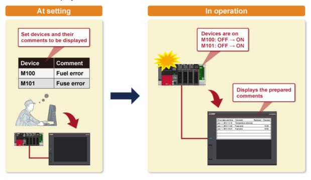
The system alarm display is a function that displays the comments preregistered in the GOT when alarms defined by the system of the GOT, controller, network, or others occur.
