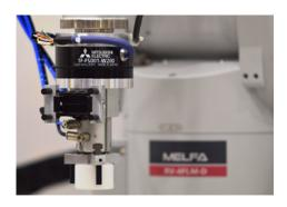
By combining Mitsubishi Electric's RV Series MELFA robots with a high-resolution force sensor and Al-enhanced force control algorithms, it is possible to create a system that mimics human interaction with robotic precision.
