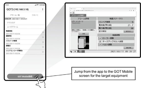
Fig. 3 Grasping equipment status and alarm history
