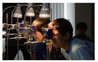
Viewing a light spectrum using a DVD spectrograph
