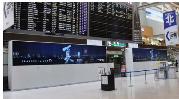
Large-scale multiple LCD screen unit (27 panels)
