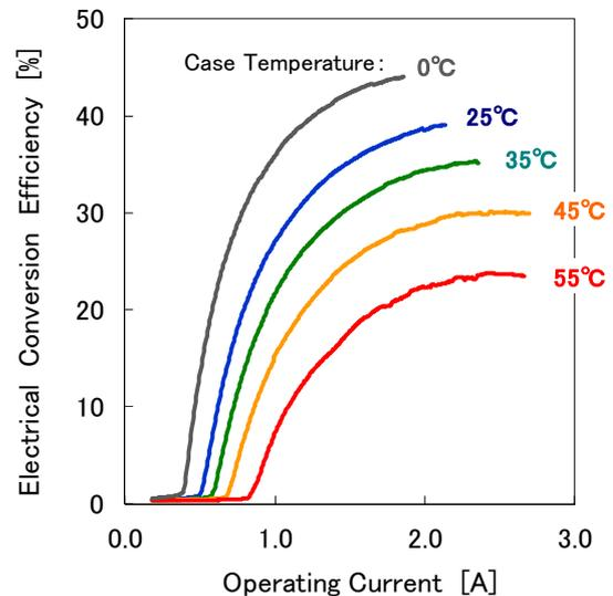
Figure 2: Conversion efficiency-current characteristics
