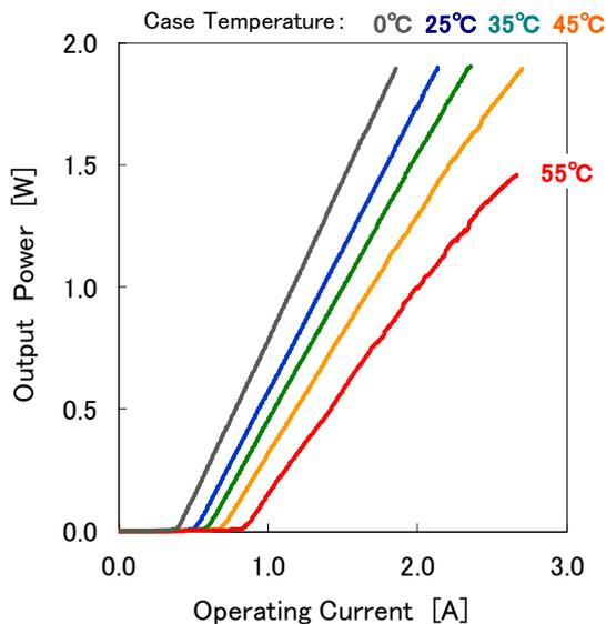
Figure 1: Power-current characteristics
