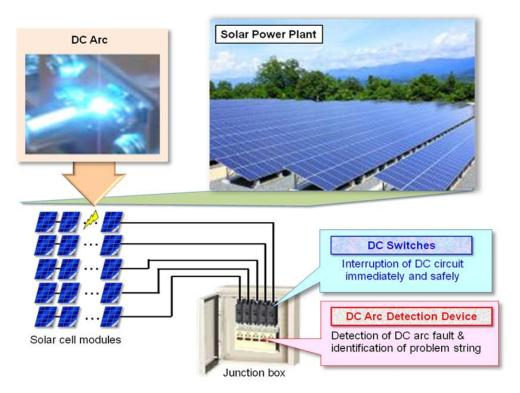
The new technology detects the DC arc fault as well as identifies the faulty circuit by monitoring sources of high-frequency current and possible deviations from normal current and voltage characteristics in solar cells.
